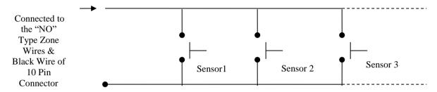
**Note:** Each Zone can be connected to one or more Sensors provided they are same type i.e., They should either be Normally Closed Type or Normally Open Type. However, different Zones can be used for different type of Sensors.
